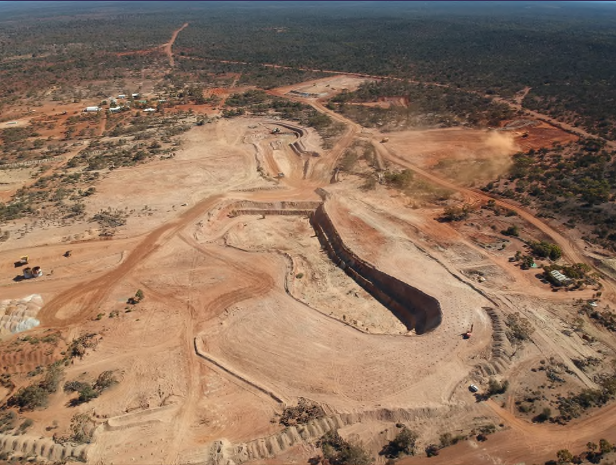
Riverina Open Pit View of Open Pit Looking South with Drill Working on Pattern (Lower Right), Stripping Topsoil from Waste Dump (Mid Right) & Establishing ROM Pad (Upper Mid)
