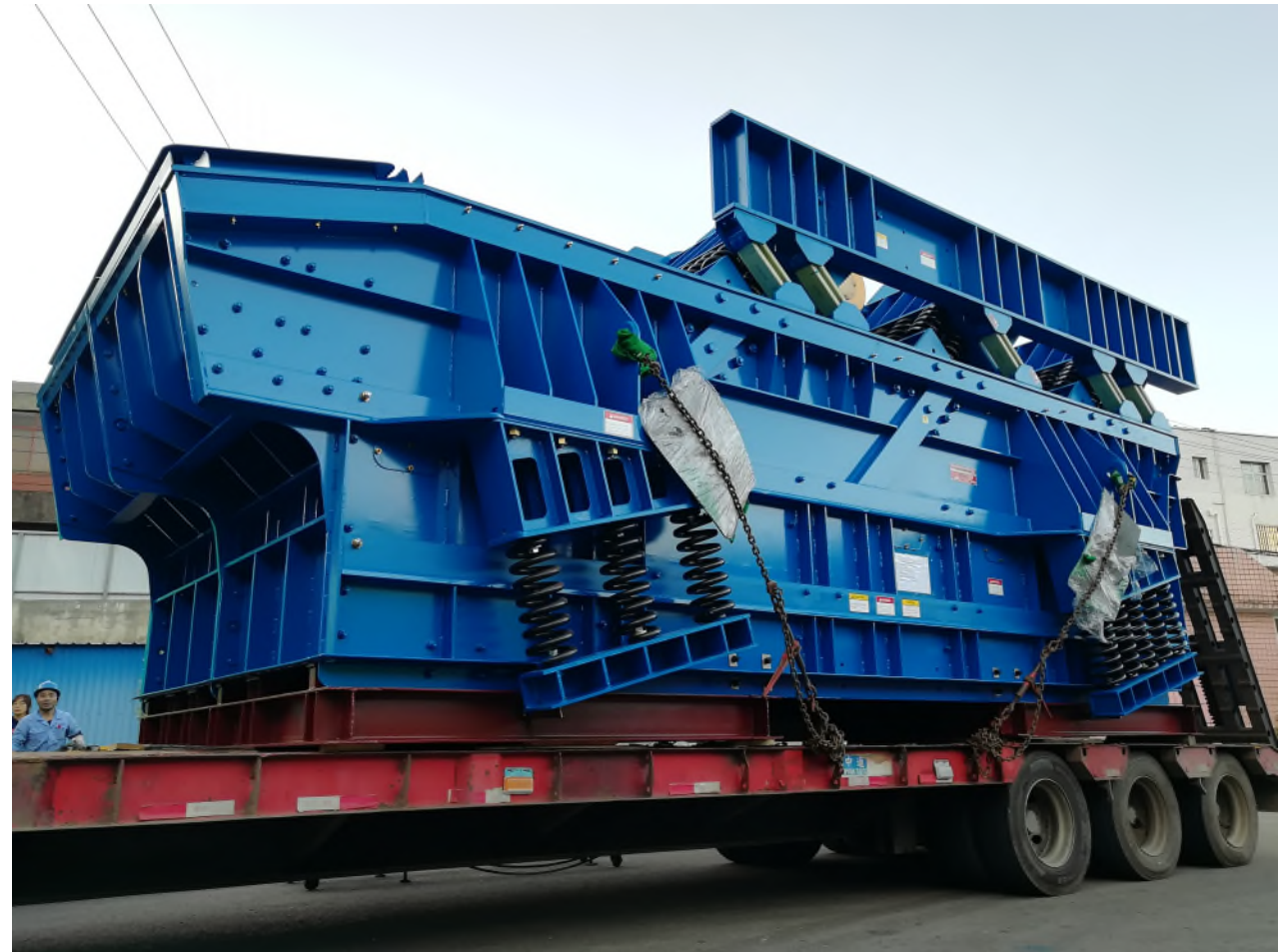
Davyhurst Process Plant New Product Screen in Transit
